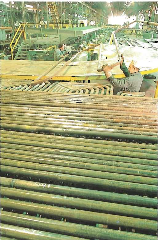
Left: Reheater elements for the Bayswater power station being produced on the CNC cold bending machine by Tubemakers of Australia Limited at Newcastle.
